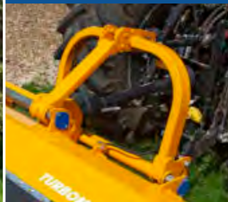
Hydraulic side shift Hydraulic offset function on all models.
