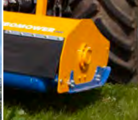
Wear skids Simple greasing and replaceable skids.
