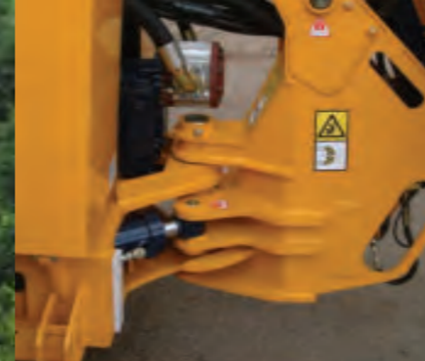
Heavy duty twin ram slew system Includes hydraulic breakout to protect machine operator.
