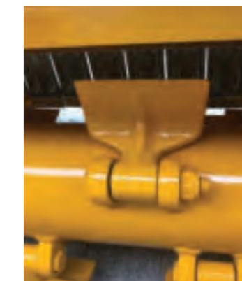
Flail type Heavy duty whale tail type flail fitted as standard.
